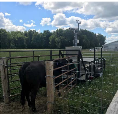
Figure 1. C-Lock Greenfeed trailers being used to measure enteric gas emissions from cows on pasture at the Ontario Beef Research Station
